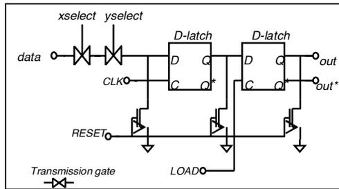
Figure 4 – Low voltage logic
