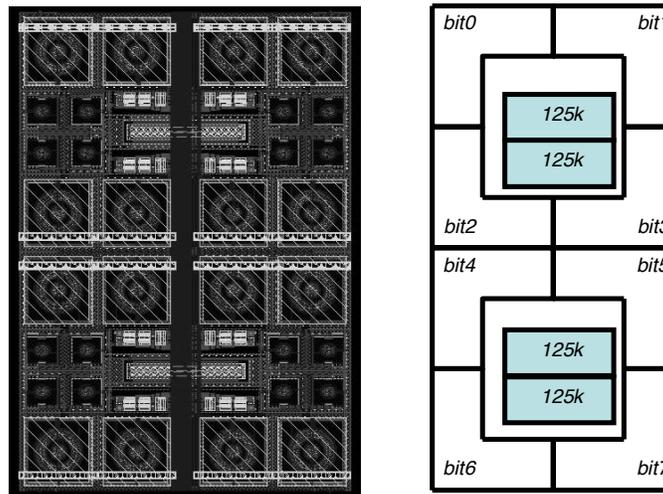
Figure 7a,b – Layout and overview of one pixel
