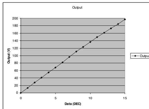
Figure 2 - Output at 200V
