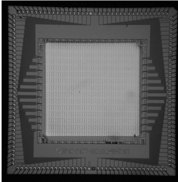
Figure 1 - 144 channel MEMS mirror
