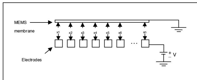
Figure 2 – Single membrane MEMS
