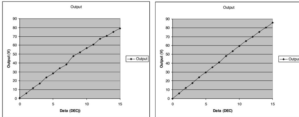
Figure 1 – Roughly tuned and correctly tuned output at 90V
