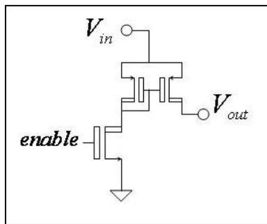
Figure 5 - High voltage switch
