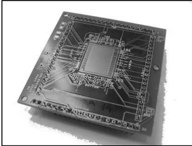
**Figure 10 - Chip carrier PCB**
